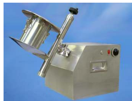
Blend-It LC005 with a 1litre Mini-Drum
