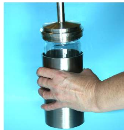
Bottle Sampler with protective Bottle Cover
