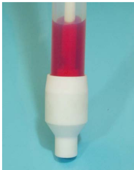
Sampler Tip Seal arrangement prevents sample from dripping
