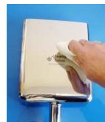
4. Clean etching area thoroughly using demineralised water
