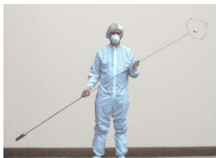
Special 3m long sampler for sampling a wet, paste using vacuum
