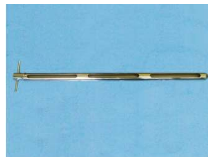
Electropolished slot sampler - this sampler was also a special length and had special slot sizes
