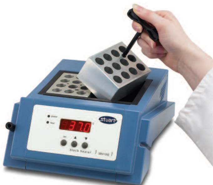
SBH130D showing block extraction tool (included)
