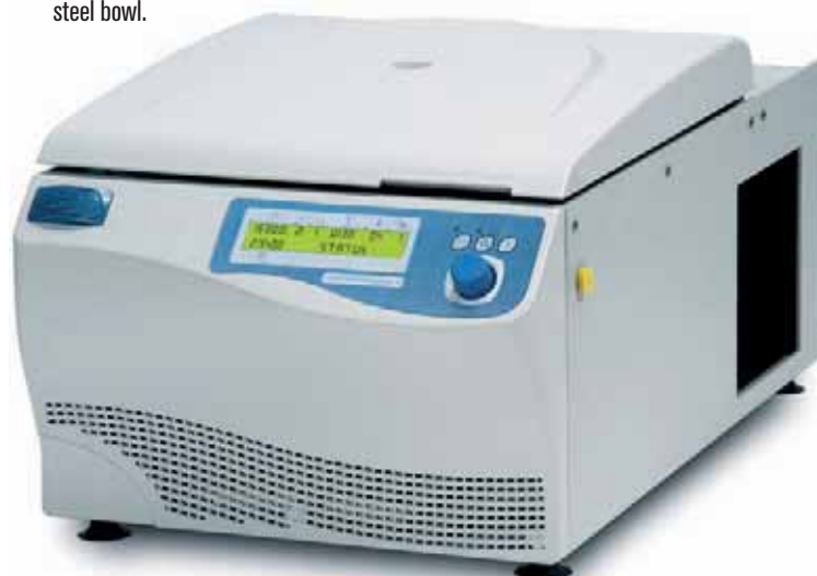
Model “Centrofriger BL-II” refrigerated, temperature range 0 °C to 30 °C.
