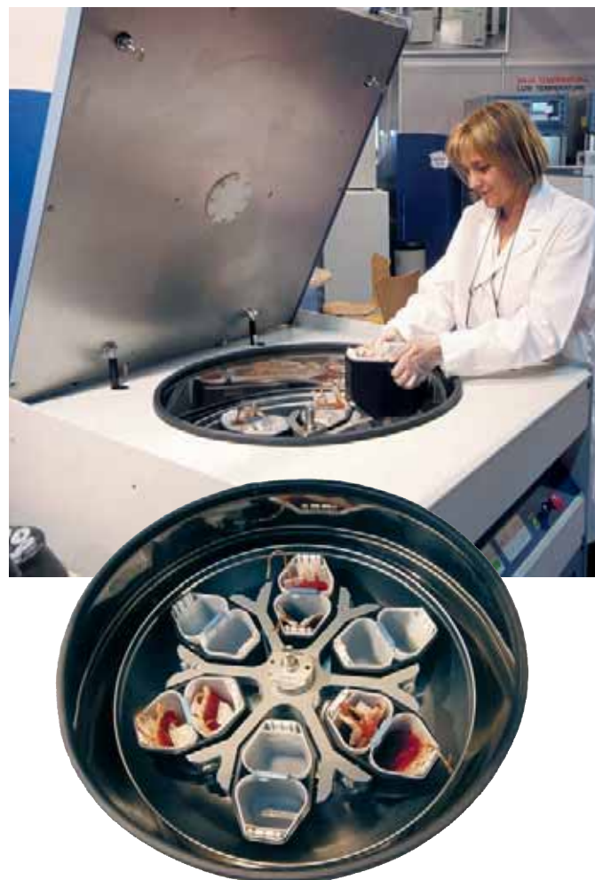
Image showing the rotor and double buckets for quad and triple blood bags of 500 and 800 ml.
