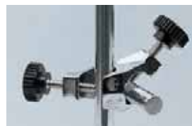
Boss head for supporting clamps. Part No. 1000069
