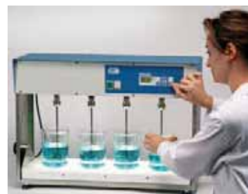
Flocculator "Flocumatic" with horizontal illumination (4 places).
