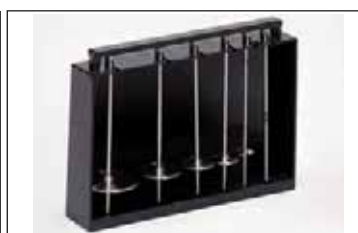
Rack of standard spindles R2, R3, R4, R5, R6 and R7: Suitable for model R.
